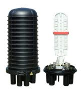
FOSC® 400 A4 Fiber Optic Splice Closure, Heat Shrink Cable sealing, two pre-installed 24-splice trays
