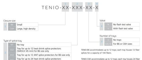
TENIO-C6H accommodates up to 12 trays; each tray houses 24 fiber splices for a capacity of 288 fibers.
