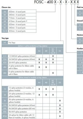
Flash test valve Pre-installed flash test valve No flash test valve Ground feedthrough G Pre-installed ground feedthrough N No ground feedthrough
