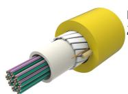
Fiber indoor cable, Plenum All-Dielectric Central Tube Rollable Ribbon, 288 fiber, Singlemode G.657.A2, Feet jacket marking, Yellow jacket color
