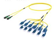
Ultra Low Loss ULL TeraSPEED® MPO(Pinned) to LC/UPC Uniboot Ruggedized fanout Cable, 24-Fiber, Plenum, 12 fiber PmP 2.0 mm Dca
