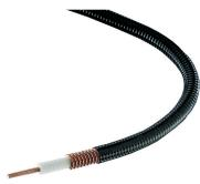
FSJ4RK-50B, HELIAX® Superflexible Foam Coaxial Cable, corrugated copper, 1/2 in, black non-halogenated, fire retardant polyolefin jacket B2ca-sla-dl-al (CPR testing is conducted annually please reference the website for latest classification)
