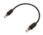
RSJ4-50 SureFlex® Jumper with interface types 7-16 DIN Male and 7-16 DIN Male with HELIAX® SureGuard weatherproofing, 6 meter
