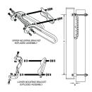
Adjustable Tilt Pipe Mounting Kit for 2.0"-4.5" (50-115mm) OD round members for panel antennas. Includes 2 clamp sets.
