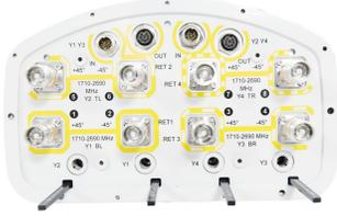
8-port sector antenna, 8x 1710–2690 MHz, 65° HPBW, 4x RET with manual override. Antenna rear wind loading 445N @ 150km/h
