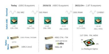
Figure 1: Chip I/O and optical integration Source: Microsoft Cloud Hardware Futures—OCP 2019
