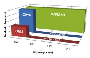
Figure 8: Bandwidth comparison of OM3, O4 and OM5 WBMMF
