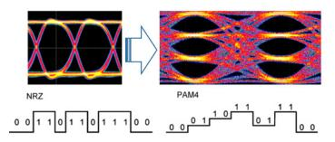
Figure 9: PAM4 modulation versus NRZ Source: Mellanox Inc., 2017
