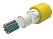
Fiber indoor cable, All-Dielectric, LSZH/Riser-Rated, Gel-Free, Central Tube Rollable Ribbon, 576 fiber, Singlemode G.657.A2, Feet jacket marking, Yellow jacket color, Cca flame rating
