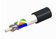
Fiber OSP cable, TeraSPEED® Single Jacket All-Dielectric, Gel-Free, Stranded Loose Tube, 72 fibers, Composite OM4 and G.652.D and G.657. Al, Feet jacket marking, Black jacket color
