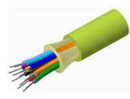
Fiber indoor cable, LazrSPEED® Low Smoke Zero Halogen Riser Distribution, 2 fiber single-unit, Multimode OM5, Feet jacket marking, Lime green jacket color, B2ca flame rating
