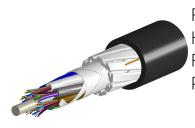
Fiber OSP cable, LightScope ZWP® Mini Single Jacket All-Dielectric, High Tensile Strength, Singlemode G.652.D and G.657.A1, 48 fiber, Gel-Filled, Stranded Loose Tube, Meters jacket marking, Black jacket color, Provides Rodent Resistance
