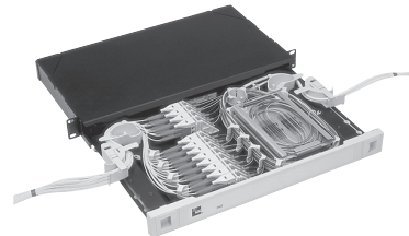
1 RU 24-Termination/Splice Drawer (Right Splice Entry)
