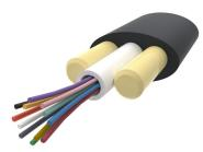
Fiber outdoor drop cable, LightScope ZWP® Self-Supporting All-Dielectric, Singlemode G.652.D and G.657.Al, 8 fiber Arid Core construction, Gel-filled, central loose tube, no ripcords, Feet jacket marking, Black jacket color
