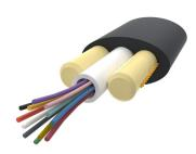
Fiber drop cable, Self-Supporting All-Dielectric, 4 fiber Arid Core construction, central loose tube, Gel-filled, Singlemode G.657.A2/B2, Meter jacket marking, Black jacket color
