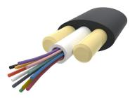
Fiber outdoor drop cable, LightScope ZWP® Self-Supporting All-Dielectric, Singlemode G.652.D and G.657.Al, 1–fiber Arid Core construction, Gel-filled, central loose tube, no ripcords, Feet jacket marking, Black jacket color
