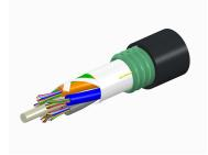
Fiber OSP cable, LightScope ZWP® Single Jacket/Single Armor, Gel-Free, Stranded Loose Tube, 24 fibers, Singlemode G.652.D and G.657.A1, Feet jacket marking, Black jacket color
