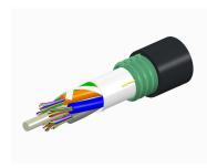
Fiber OSP cable, LightScope ZWP® Single Jacket/Single Armor, Gel-Free, 48 fibers, Stranded Loose Tube, Singlemode G.652.D and G.657.A1, Feet jacket marking, Black jacket color
