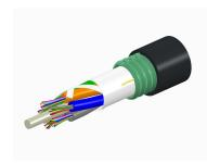
Fiber OSP cable, LightScope ZWP® Single Jacket/Single Armor, 60 fibers, Gel-Free, Stranded Loose Tube, Singlemode G.652.D and G.657.A1, Feet jacket marking, Black jacket color
