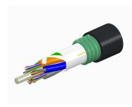
Fiber OSP cable, LightScope ZWP® Single Jacket/Single Armor, 288 fiber, Gel-Free, Stranded Loose Tube, Singlemode G.652.D and G.657.A1, Feet jacket marking, Black jacket color
