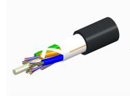
Fiber OSP cable, LightScope ZWP® Single Jacket All-Dielectric, 12 fiber, Gel-Free, Stranded Loose Tube, Singlemode G.652.D and G.657.A1, Feet jacket marking, Black jacket color
