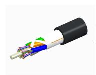
Fiber OSP cable, LightScope ZWP® Single Jacket All-Dielectric, 12 fiber, Gel-Free, Stranded Loose Tube, Singlemode G.652.D and G.657.Al, Meter jacket marking, Black jacket color
