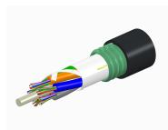
Fiber OSP cable, LightScope ZWP® Single Jacket/Single Armor, 72 fiber, Gel-Free, Stranded Loose Tube, Singlemode G.652.D and G.657.Al, Meters jacket marking, Black jacket color
