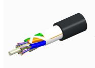
Fiber OSP cable, LightScope ZWP® Single Jacket All-Dielectric, 72 fiber, Gel-Free, Stranded Loose Tube, Singlemode G.652.D and G.657.A1, Meter jacket marking, Black jacket color
