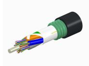
Fiber OSP cable, LightScope ZWP® Single Jacket/Single Armor, 156 fiber, Gel-Free, Stranded Loose Tube, Singlemode G.652.D and G.657.A1, Feet jacket marking, Black jacket color
