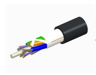
Fiber OSP cable, LightScope ZWP® Single Jacket All-Dielectric, Gel-Free, Stranded Loose Tube, 4 fiber, Singlemode G.652.D and G.657.Al, Meter jacket marking, Black jacket color
