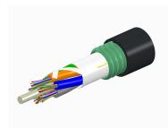
Fiber OSP cable, LightScope ZWP® Single Jacket/Single Armor, 192 fiber, Gel-Free, Stranded Loose Tube, Singlemode G.652.D and G.657.Al, Meters jacket marking, Black jacket color
