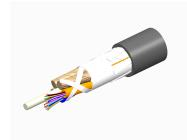
Fiber indoor/outdoor cable, LightScope ZWP®, Single Jacket All-Dielectric, Plenum Rated, 144 fiber, Singlemode G.652.D and G.657.Al, Gel-Free, Stranded Loose Tube, PVDF jacket, Meters jacket marking, Black jacket color
