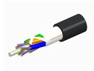
Fiber OSP cable, LightScope ZWP® Single Jacket All-Dielectric, 132 fiber, Gel-Free, Stranded Loose Tube, Singlemode G.652.D and G.657.Al, Meters jacket marking, Black jacket color
