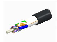
Fiber OSP cable, LightScope ZWP® Single Jacket All-Dielectric, 168 fiber, Gel-Free, Stranded Loose Tube, Singlemode G.652.D and G.657.Al, Meters jacket marking, Black jacket color
