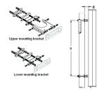
Adjustable Tilt Pipe Mounting Kit for 2.362"-4.5" (60-115mm) OD round members for panel antennas. Includes 2 clamp sets.
