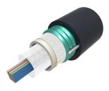
Fiber OSP cable, Steel Armored, Arid-Core, Dry Central Tube Ribbon, 144 fiber, Singlemode G.657.A2, Feet jacket marking, Black jacket color
