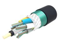
Fiber OSP cable, Steel Armored, Gel-Filled Loose Tube Ribbon, 720 fiber, Singlemode G.657.A2, Feet jacket marking, Black jacket color
