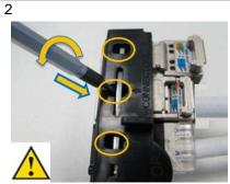
...insert the screwdriver through the selected opening and press the "jack latch" at same time that rotates it...
