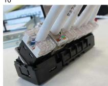
Pre-insert the "sub-assy. metal frame" (as shown in fig.3) into the "holder".
