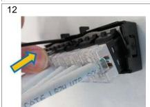
Once pre-inserted, pivot the "subassy metal frame" while pushing it toward the "top surface" of the holder
