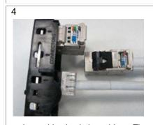
...by pushing back the cable.... The single cable assembly is completely out.
