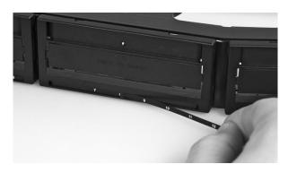
2.1. Mount the patch panel onto the cabinet / rack. Insert the port ID labels.
