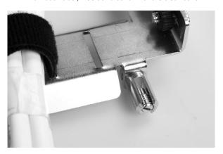
2.7. Install the grounding bolt at the back of the panel.
