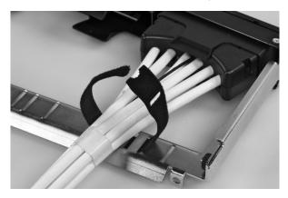
2.5. After installation of the cassettes, bring the cable management bar back into original position, Tighten the knurled nuts. Secure cable bundle, using velcro straps (PN 1375253-2), to the cable management bar.
