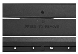
2.2. Remove cover, for those ports which will be used, by pressing on the "press to remove" area.
