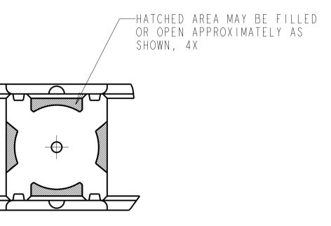
DETAIL A ALTERNATE CENTER BRACE CONFIGURATION
