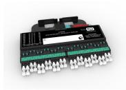
FACT® MPO Module, right sided, LC at front side, 1x24 fiber MPO at rear side, ULL multimode OM4, wiring method A
