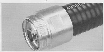
Add a thin coating of silicone grease to the outer surface of the threaded gasket and the inner surfaces of the splice nut, splice body, and threaded body. Slide the splice nut onto one cable and then screw the splice body onto the outer conductor so that about 1/8" (3 mm) of the conductor protrudes. Wipe off any silicone grease from the protruding outer conductor. Install the threaded body onto the other cable in the same way as the splice body.
