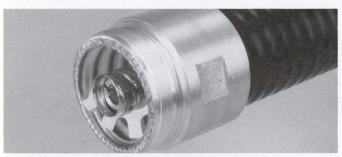
Pull the dielectric spacer out and trim it flush with the outer conductor tabs. Then file the inner conductor to within 1/8" (3 mm) of these tabs and remove any loose particles. Screw the inner stub into the conductor far enough to allow cutting notches in the conductor.
