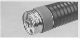
Turn the threaded gasket inside out and stretch it over the end of the cable. Then flip the gasket over and screw it into position against the cable jacket.
