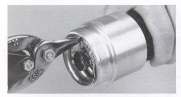
Push in the end of the dielectric spacer to allow for conductor tab cutting. Cut the outer conductor at 3/16" (5 mm) intervals to form tabs. Bend and gently flatten the tabs against the splice body and the threaded body using the plastic rod and mallet, but do not thin the copper. File off any burrs and then clean the tabs with solvent.
