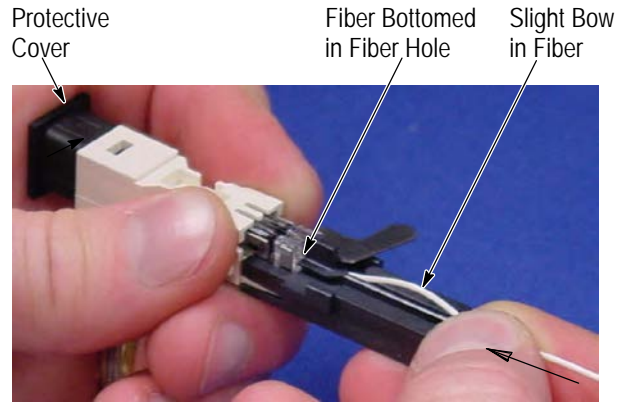
Insert Fiber into Fiber Hole
