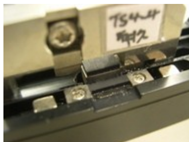
Fig.12 Blade slide and fiber bending pillow, 50000 times
