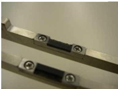
Fig.11 Fiber holding lever, 50000 times
