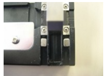
Fig.7 Blade slide guide, 10000 times
