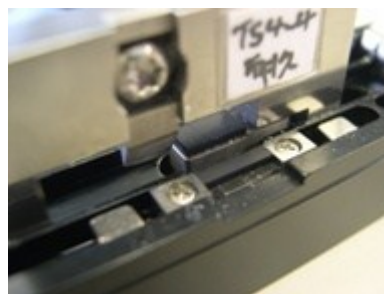
Fig.6 Blade slide and fiber bending pillow, 10000 times
