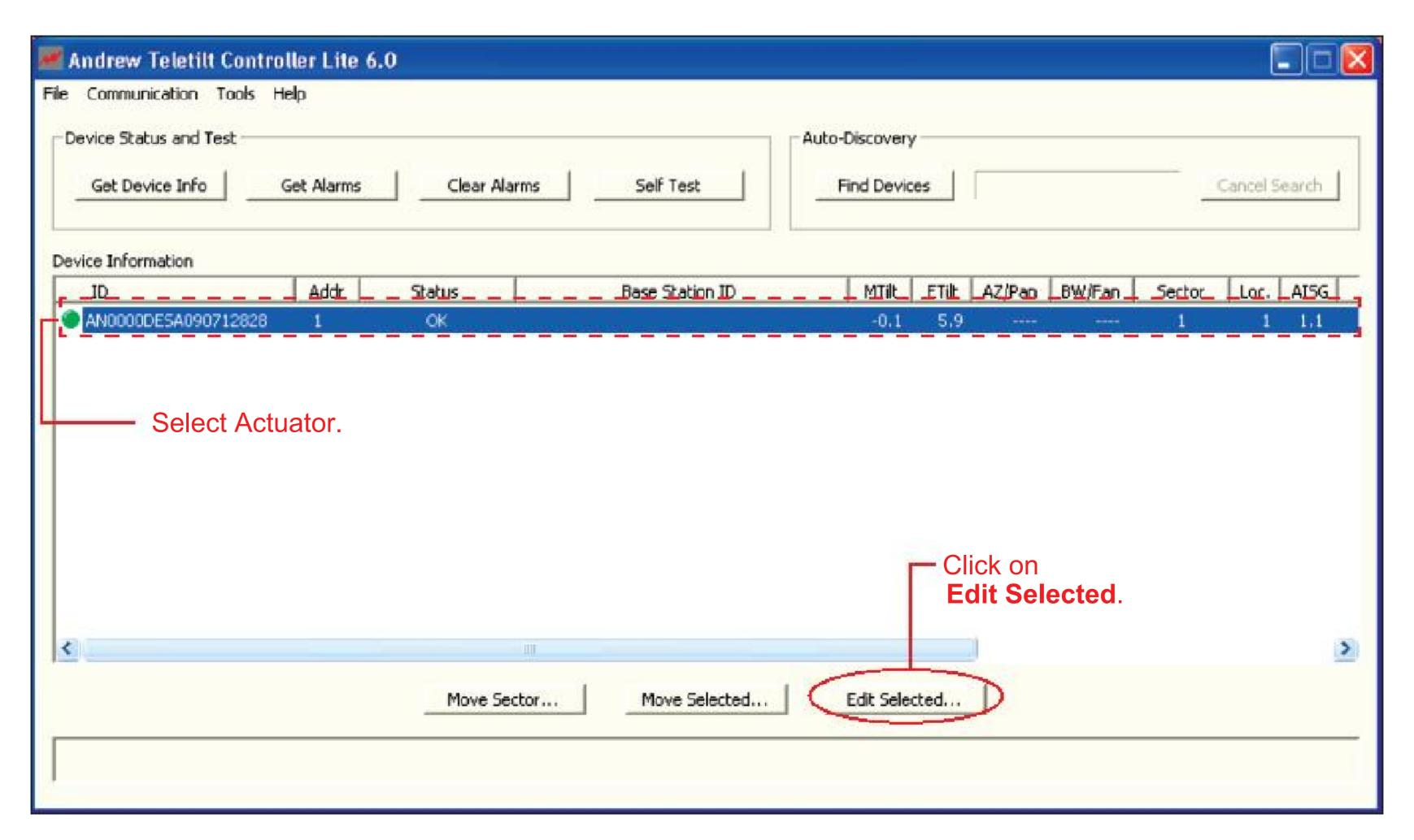
Figure 3-3. Selecting Actuator In A RET Antenna System.
