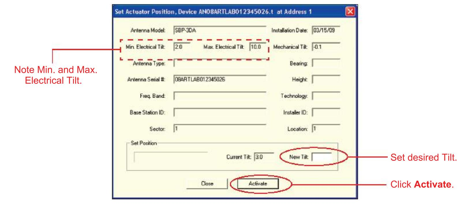
Figure 3-6. Adjusting Tilt To Minimum And Maximum Settings.
