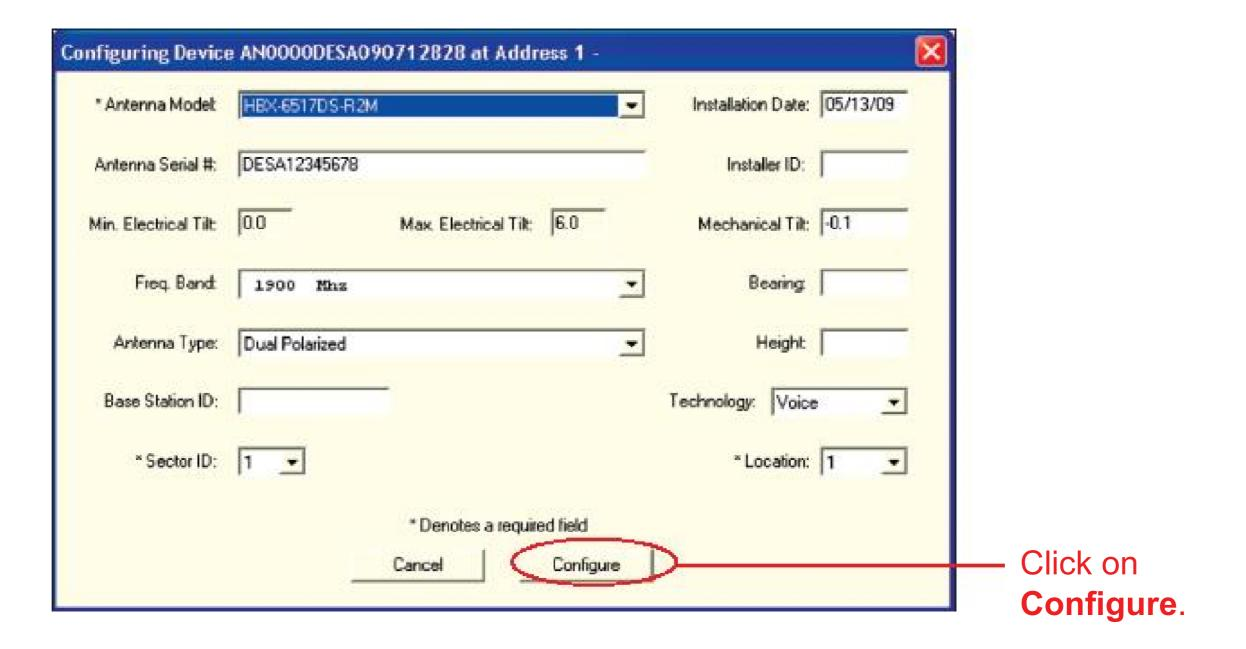
Figure 3-4. Configuring A Selected Device Prior To Operations.
