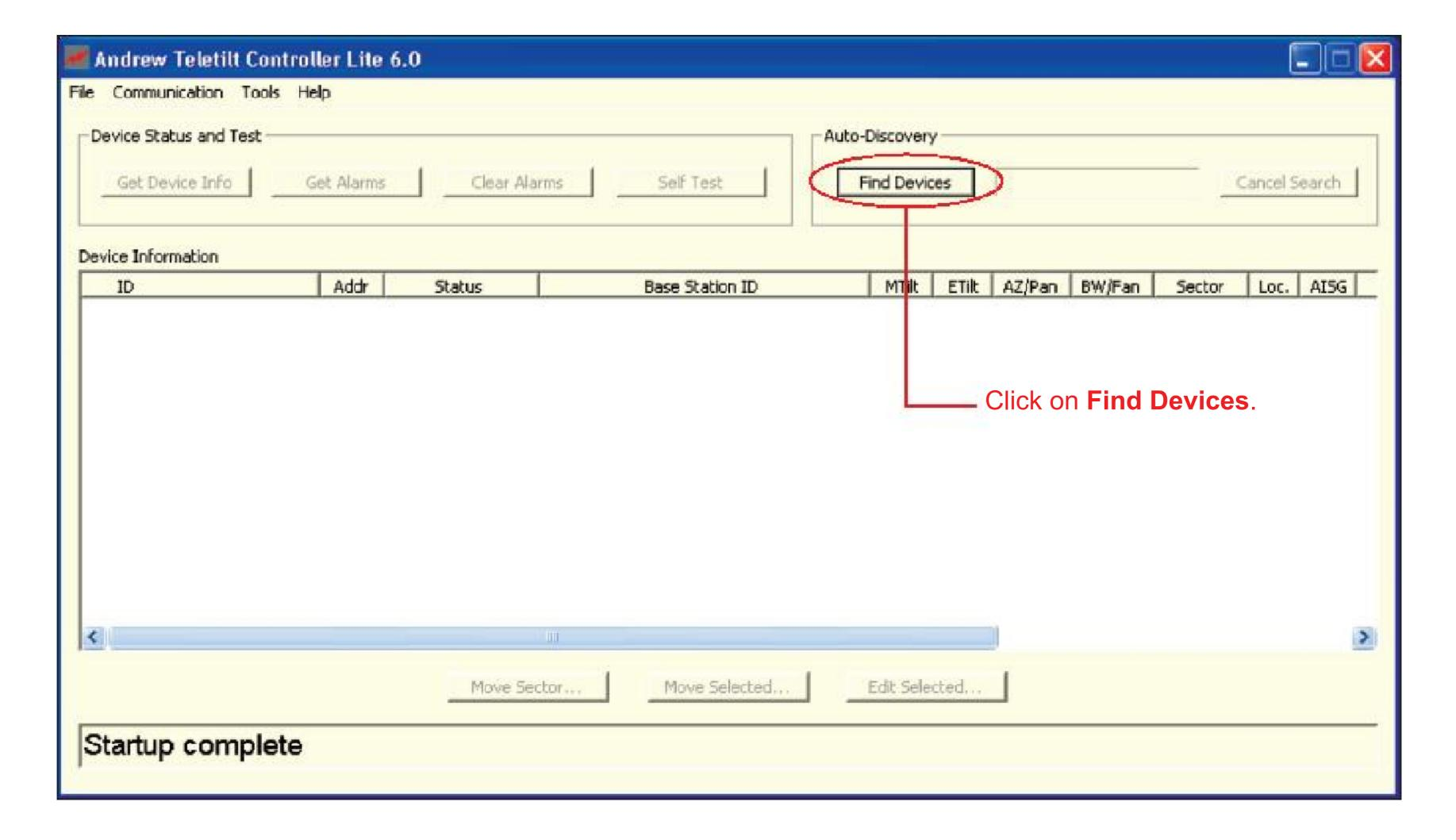
Figure 3-2. Main Startup Screen Ready For Device Search.
