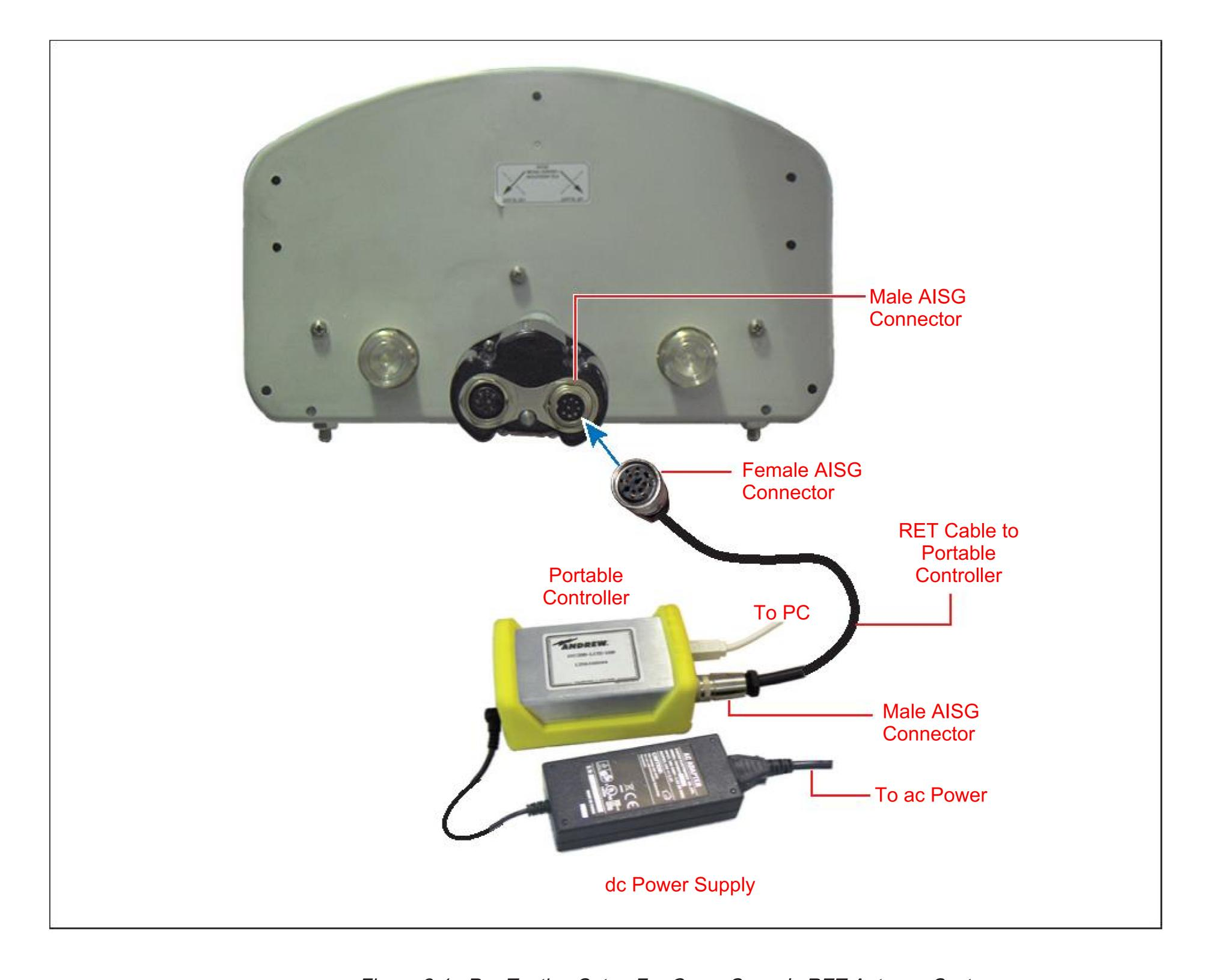
Figure 2-1. Pre-Testing Setup For CommScope's RET Antenna System.
