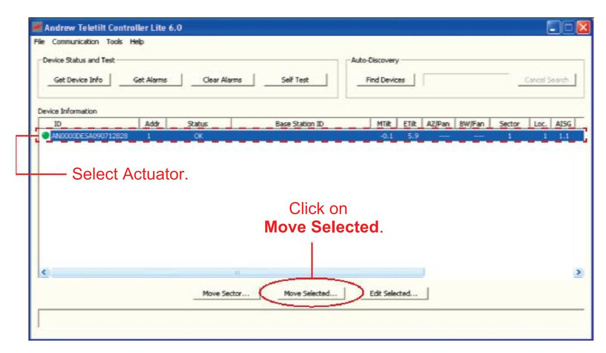
Figure 3-5. Selecting The Actuator To Be Tested.
