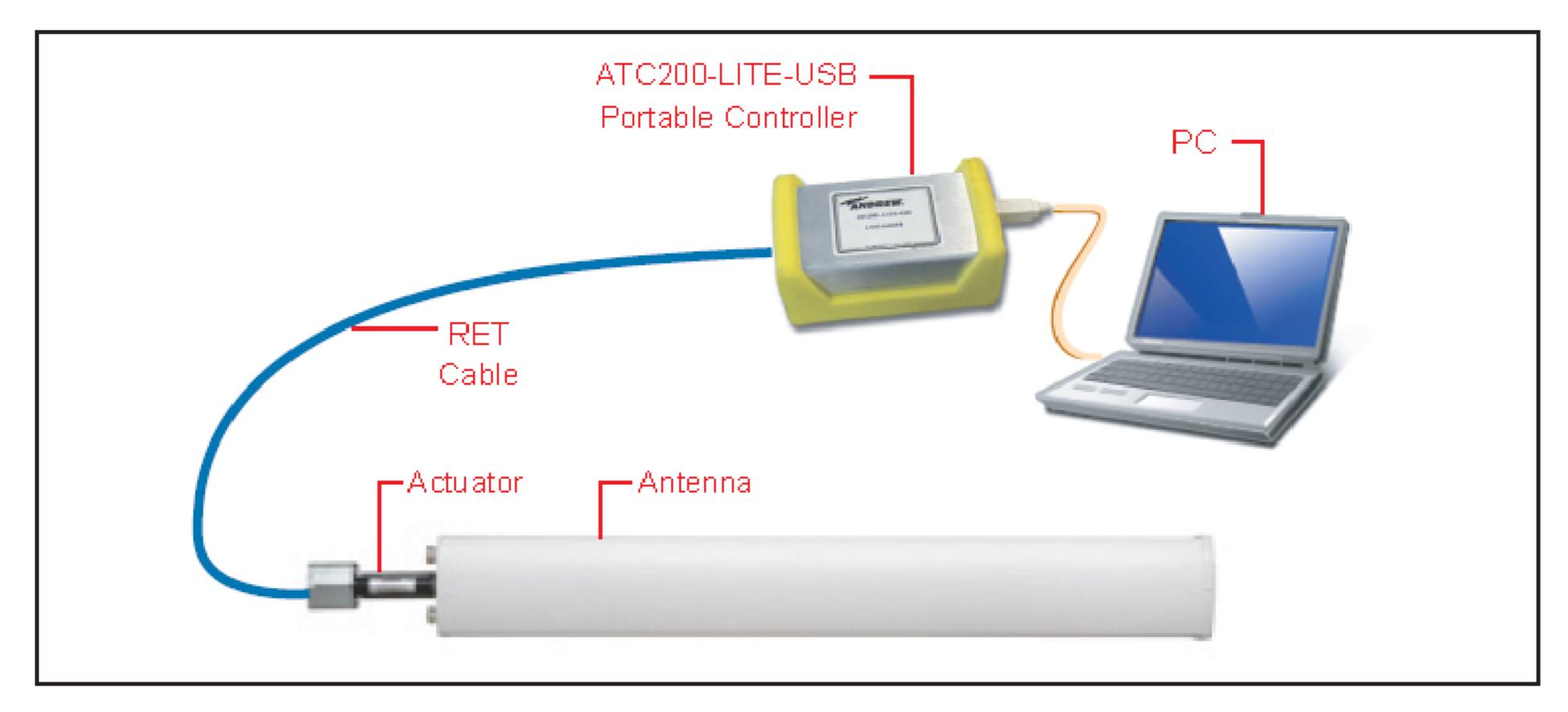
Figure 1-1. Pre-Testing Setup For CommScope RET Antenna System.
