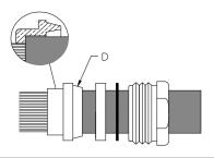
Fold braid around part D and comb braid as shown, the braid should be straight and equally spaced after comb.
