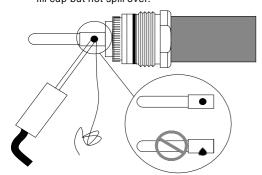
The cable attachment must be straight and aligned with the hole of connector inner contact. Insert the cable attachment into connector body until stopped; the center conductor must be inserted into the hole of insulator. Tighten the connection to the torque value of 60-80 lb-in (6.8-9.0 Nm). Note: Do not turn connector body, turn cable attachment.
