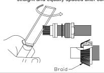
Cut off the redundant braid as shown.
