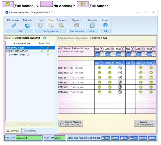
Figure 12 Antenna Sharing Access Level available for the chosen Antenna Model Online Mode
