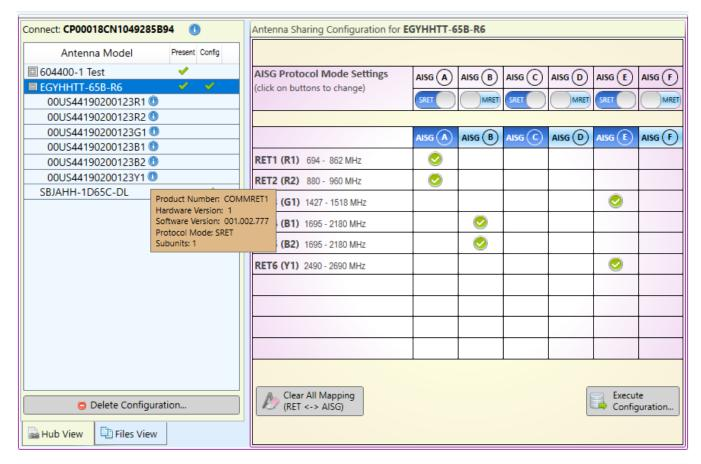
Figure 11 Configuration for Antenna Model 'EGYHHTT-65B-R6' depicting Scenario 4. Mixed RETs mapping.
