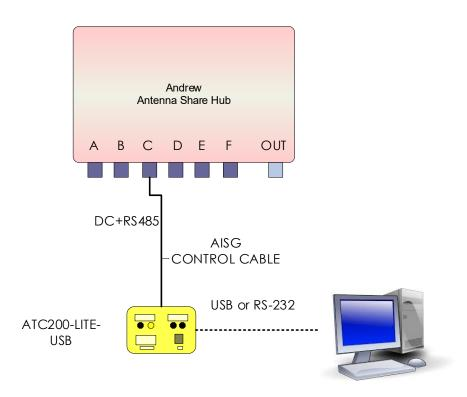
Figure 6 ATC200-LITE-USB connected to ANDREW Antenna Sharing Hub on control port C.
