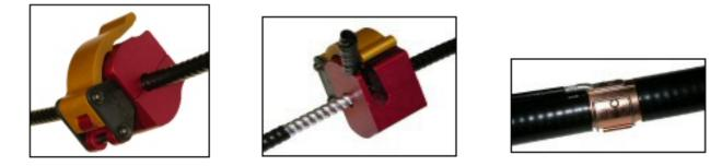
NOTE: In cases where cable variations cause strip blade to come in contact with the aluminum sheath, the spring washer stored under the screw head may be installed under the jacket strip blade. (Hex key is enclosed with tool.)
