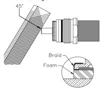
The cable attachment must be straight and aligned with the hole of connector inner contact. Insert cable attachment into connector body until stopped; the center conductor must be inserted into the connector inner contact fingers. Tighten the connection to the torque value of 60-80 lb-in (6.8-9.0 Nm). Note: Do not turn connector body, turn cable attachment.
