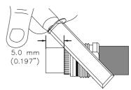
Chamfer the center conductor at a 45° angle.
