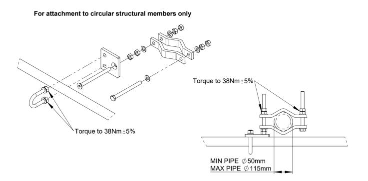
Struts must be attached to a circular structural member capable of supporting 2704N in line with TIA-222.
