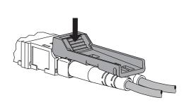
Press down on grip area of removal tool to release lock
