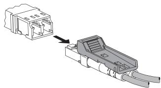
3 Pull connectors out of adapter then disengage removal tool
