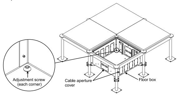
**Note**: Planning and organizing equipment to be installed in floor box prior to completing box installation will be beneficial. Equipment mounting rails in box can be angled or adjusted to accommodate different size equipment. See Steps 3 and 4 for instructions before completing box installation.
