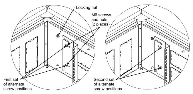
**Note**: Using M6 screws and nuts provided, the equipment mounting rails may be repositioned to suit deeper equipment. This must be done prior to installing the floor box into the raised floor.
